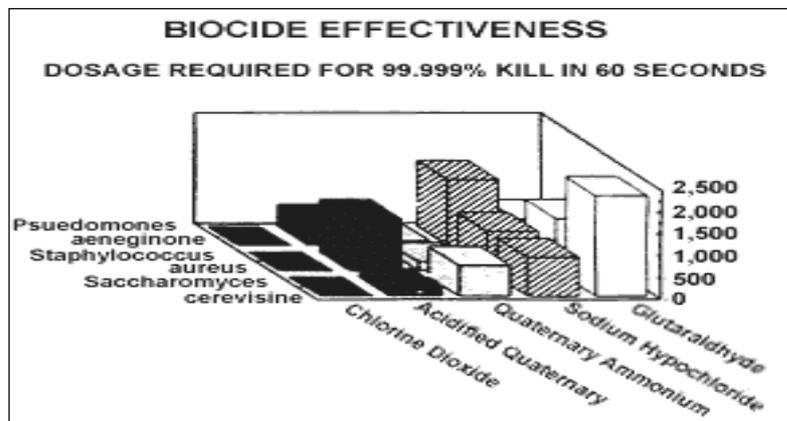
In this graph the disinfectants like Quaternary Ammonium Compounds, Sodium Hypochlorite and Glutaraldehyde requires the dose of more than **500 ppm** to bring about 5-log reduction in viable bacteria at 60 seconds contact time. It is clear from this figure that chlorine dioxide reacts very rapidly, achieving a 99.999% reduction in viable bacterial cells in one minute at low dosage when compare to other disinfectants.
